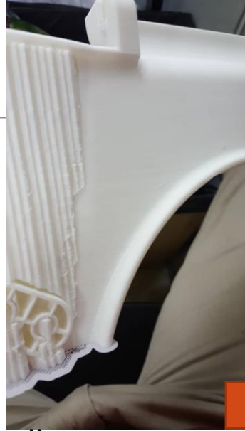
Excess printing jig needs to be removed
