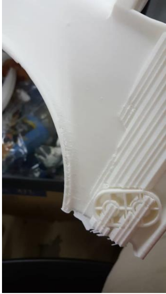
Excess printing jig needs to be removed
